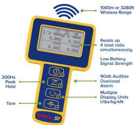
Decades of development into this product include many stand out features such as SP's unique strain gauging method that helps compensate for wire rope torque when the Radiolink is loaded. The Radiolink plus tension load cell can also be used in combination with Crosby | Straightpoint 'INSIGHT' high speed wireless data logging software allowing for simultaneous control, display and real time data logging of up to 126 Crosby | Straightpoint wireless load cells.
