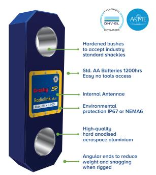
Radiolink plus is designed to be rigged with Crosby standard shackles - DNV-GL type approved wireless tension load cell capable of weighing and dynamic load monitoring in capacities from 1t to 500t – from stock with an ATEX and IECEx version available for hazardous areas, zones 0, 1 & 2.
