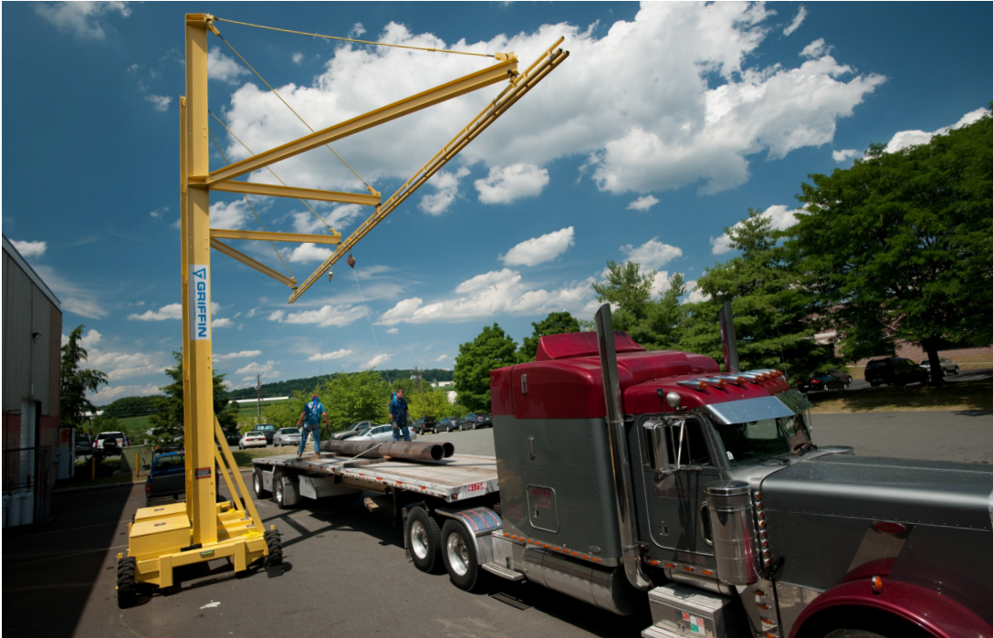
Mobile Rigid Rail Fall Protection System 22ft under rail, 45ft long.
