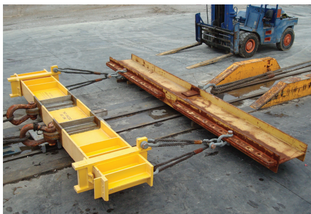
235 ton load test of a 20 ft. (yellow) turbine-lifting spreader beam
