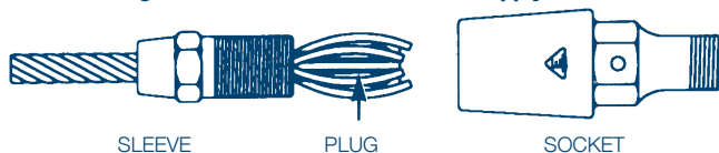
Plug driven in and strands closed to apply socket.
